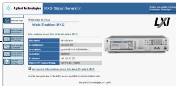
The FTP access button opens a window that displays the signal generator's memory catalog files.
